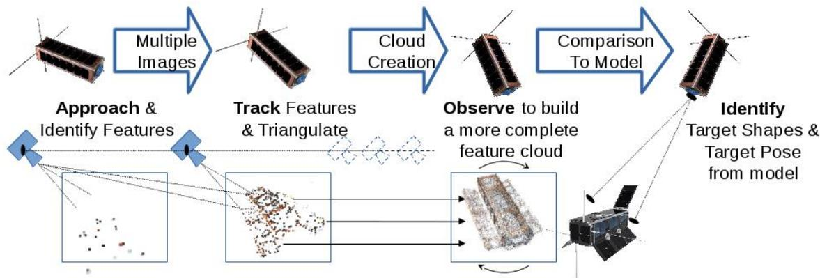
Figure 10: Illustration of sequential reconstruction of a target satellite from multiple perspectives of a chaser satellite.
