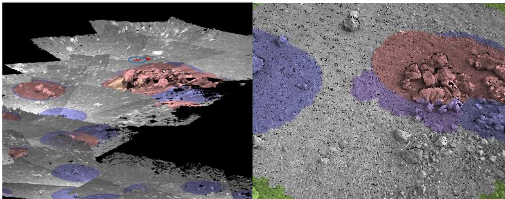
Figure 1: Illustration of Digital Terrain Maps built with a sequence of stereovision data. A luminance value has been associated to each cell (colors encode a notion of traversability, out of the scope of the DFPC)
