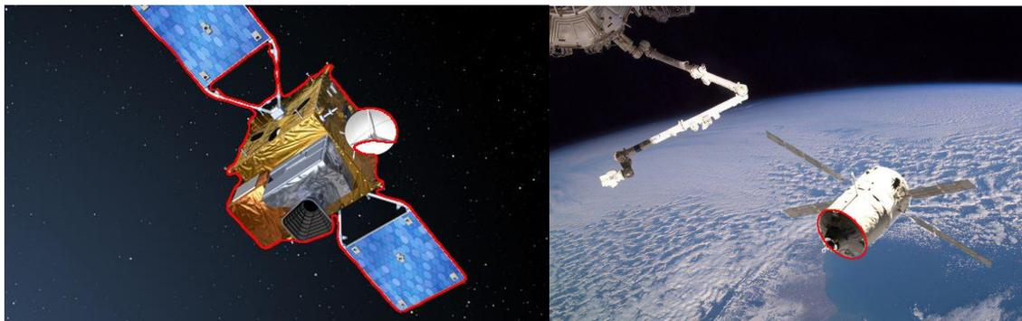
Figure 8: Illustration of the target satellite localization at mid-range (left, the full target model is used to localize it) and short range (right, only parts of the target model are used to localize it).
