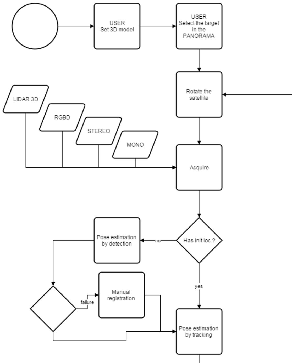
Figure 9: Generic flow chart of the satellite state estimation
