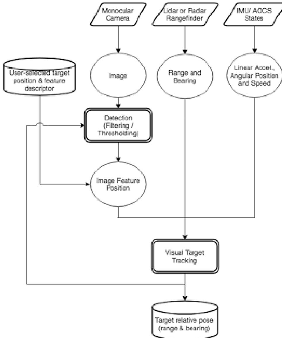
Figure 6: Overview of the detection, range and bearings estimate of the target satellite at far range
