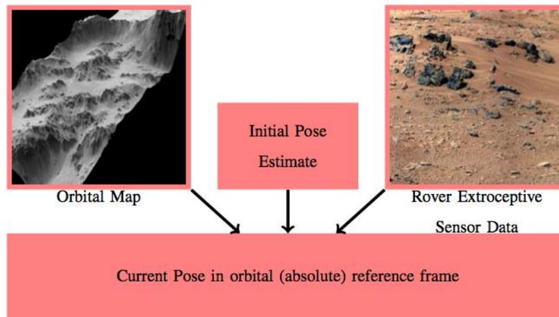
Figure 12: A Graphical Illustration of the Pose Estimation Problem
