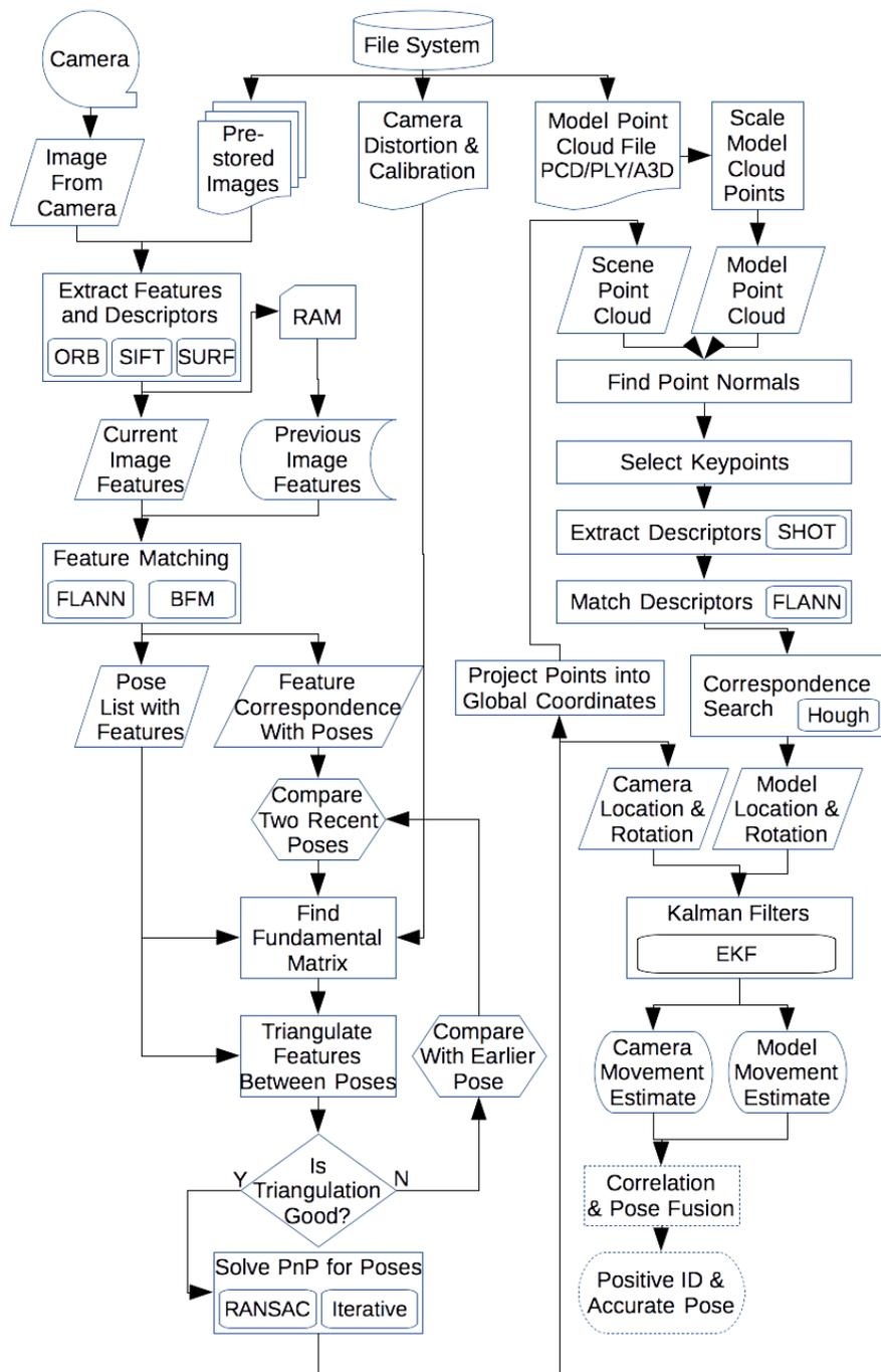
Figure 11: Generic flow chart of 3D target reconstruction and tracking using 3D model-based point cloud recognition
